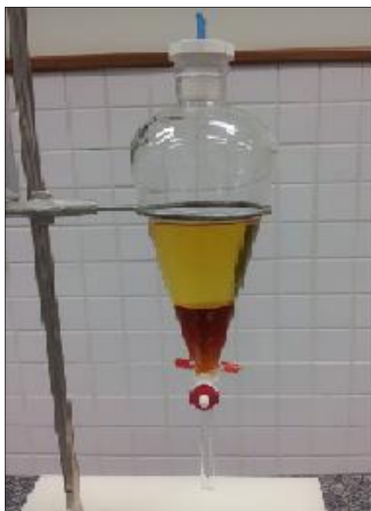
Fig 2: Separation of Biodiesel using separating funnel
