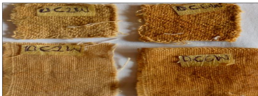
Fig 6: Cotton and wool fabrics dyed with dye extract and test for wash fastness
