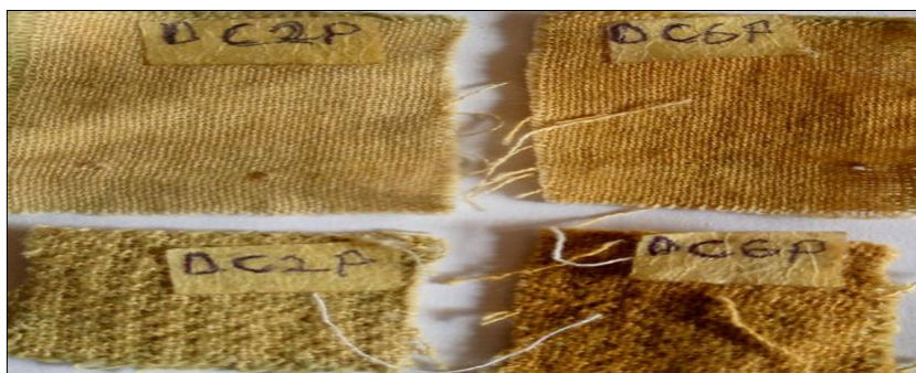
Fig 7: Cotton and wool fabrics dyed with dye extract and test for perspiration fastness
