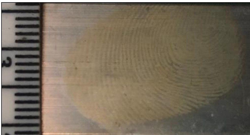
Fig 1: Photographic image of a developed latent fingerprint on an aluminum surface, exhibiting a quality score of 4. The fingerprint was obtained using a PCS gel prepared with a 1:1:1 ratio consisting of 5 mL of 5% w/v KMnO 4 solution, 5 mL of 1% w/v CaCl 2 solution, and 5 g of silica powder.
